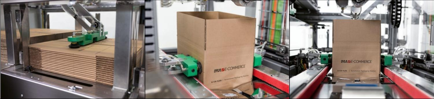
The E-CO Flex boasts the market's widest case magazine, capable of accommodating up to 12 distinct box sizes. This intelligent system efficiently selects the most suitable box size based on the volume of each individual order to be packed.
