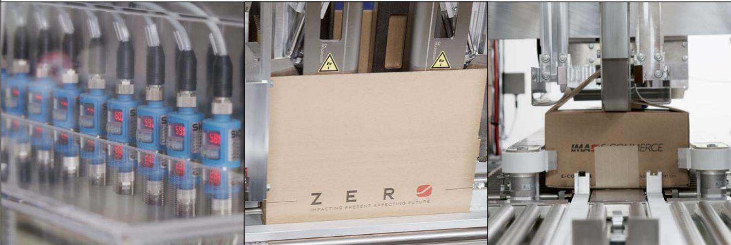
Upon inserting the open-faced case into the closing module, a bank of ultrasonic sensors meticulously measures the remaining void within the box.
