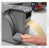
Push lever to dispense tape to desired length (Additional pushes may be required).
