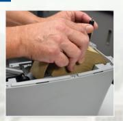
Remove cover to insert tape, then feed tape through slot.
