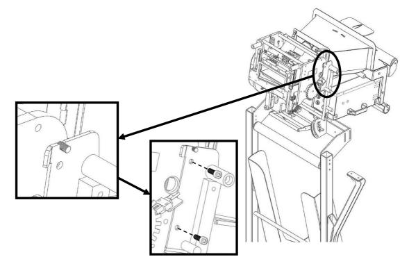
Install the Running Gear and Cutter Modules -2 Figure 4-15
