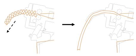
**1.2** Press the *Gear Reverse Key* for 2~3 times to loosen the jam, then press the Gear Forward Key for once to output paper.
