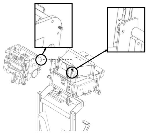
Install the Running Gear and Cutter Modules -1 Figure 4-14
