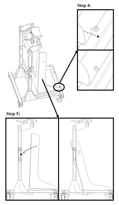
Install the Floor Stand – Step 4 & Step 5 Figure 4-6
