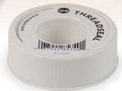
**Thread Seal Tape** is made from a 100% virgin PTFE film. Withstands alkalies, acids, hydro-carbons, solvents, refrigerants, gases and steam. Meets MIL-T-27730-A. Contains no lead or toxic chemicals. Not suited for petroleum products.
