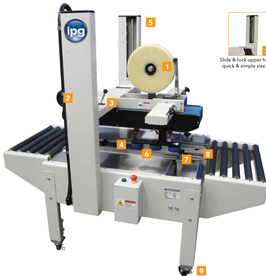
2 1/2 HP lower and 1/4 HP upper gear motors to process cases up to 85 lbs.
