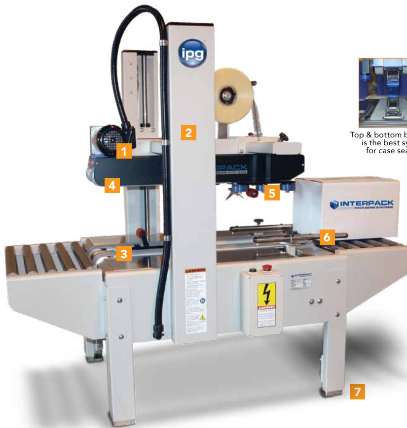
1 1/2 HP lower and 1/4 HP upper gear motors to process cases up to 85 lbs.
