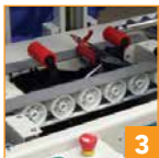
Top & bottom belt drive with belt over roller technology
