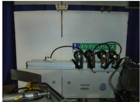
the separation of blank cases from each other to **Figure 4-10 Vacuum Cup Mechanism**
