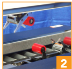
Offset tape heads process 2" high cases
