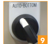
Top & bottom or bottom only seal operation modes
