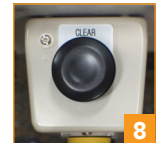
"Clear" button for jams & replacing bottom tape roll (Opposite Side of Machine)
