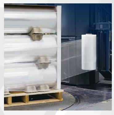
A real-world example of stretch film performance comes from a customer who replaced their original film with <u>IPG's G7</u> Ultra High-Performance film. Without changing their equipment, they increased load retention from 12.7 lbs to 15.0 lbs on one machine and from 18.3 lbs to 22.6 lbs on another.
