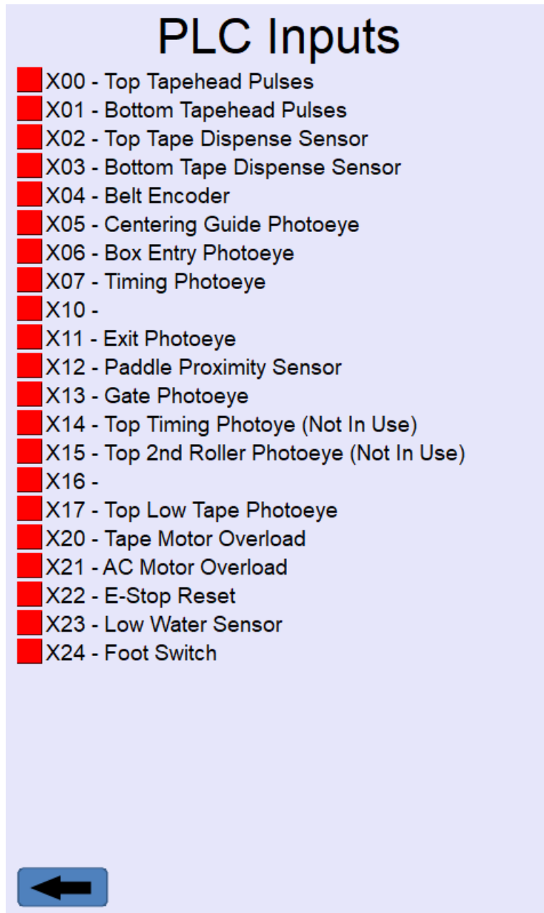
Figure 59: HMI PLC Input Screen
