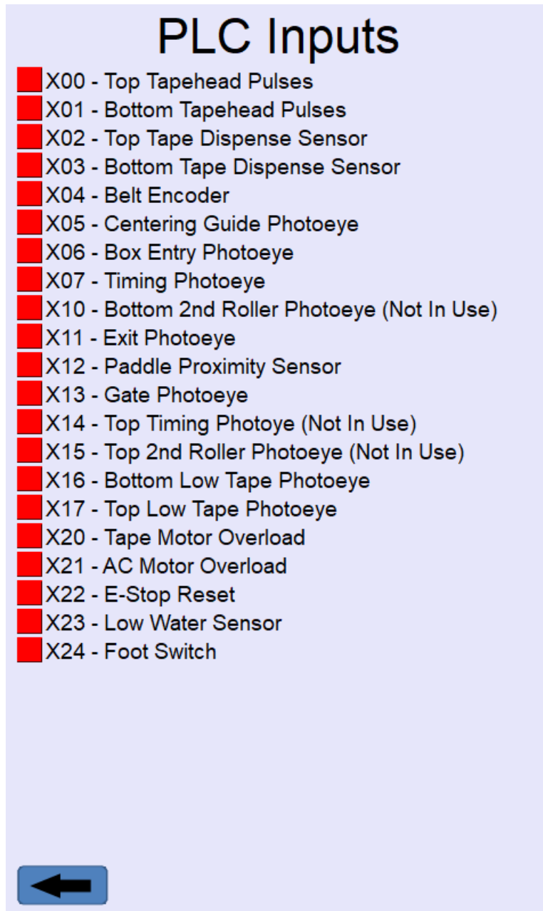
Figure 67: HMI PLC Input Screen
