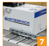
7 Horizontal centering guides with rollers
