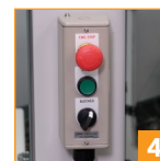
4 "Blocked" button for jams replacing bottom tape roll
