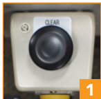
"Clear" button for jams & replacing bottom tape roll (opposite side of machine)
