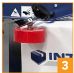
Standard top squeezers compress the major flaps prior to taping for a more secure seal
