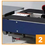
Bottom belt drive processes heavier cases
