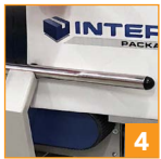
Arcing self-centering guides make case size setup simple
