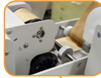
Powered tape unwind
