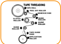
Threading diagram delivers easy tape roll change
