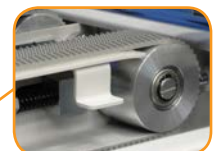
Self-tensioning & self-tracking drive belts simplify belt replacement
