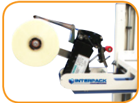
Tip-up tape head simplifies roll replacement
