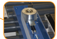
Self-tensioning & tracking side drives simplify belt replacement
