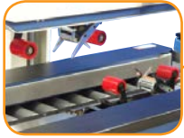
Offset tape heads process 2" high cases
