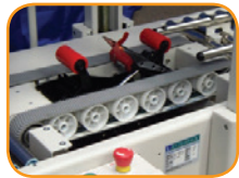
Top & bottom belt drive with belt over roller technology
